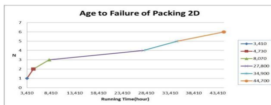
Figure 3 – Life Data of HP Packing Cylinder 2D at Each Repair
